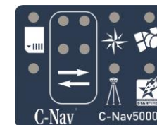
Figure 2: C-Nav5000 LED Indicator Panel
